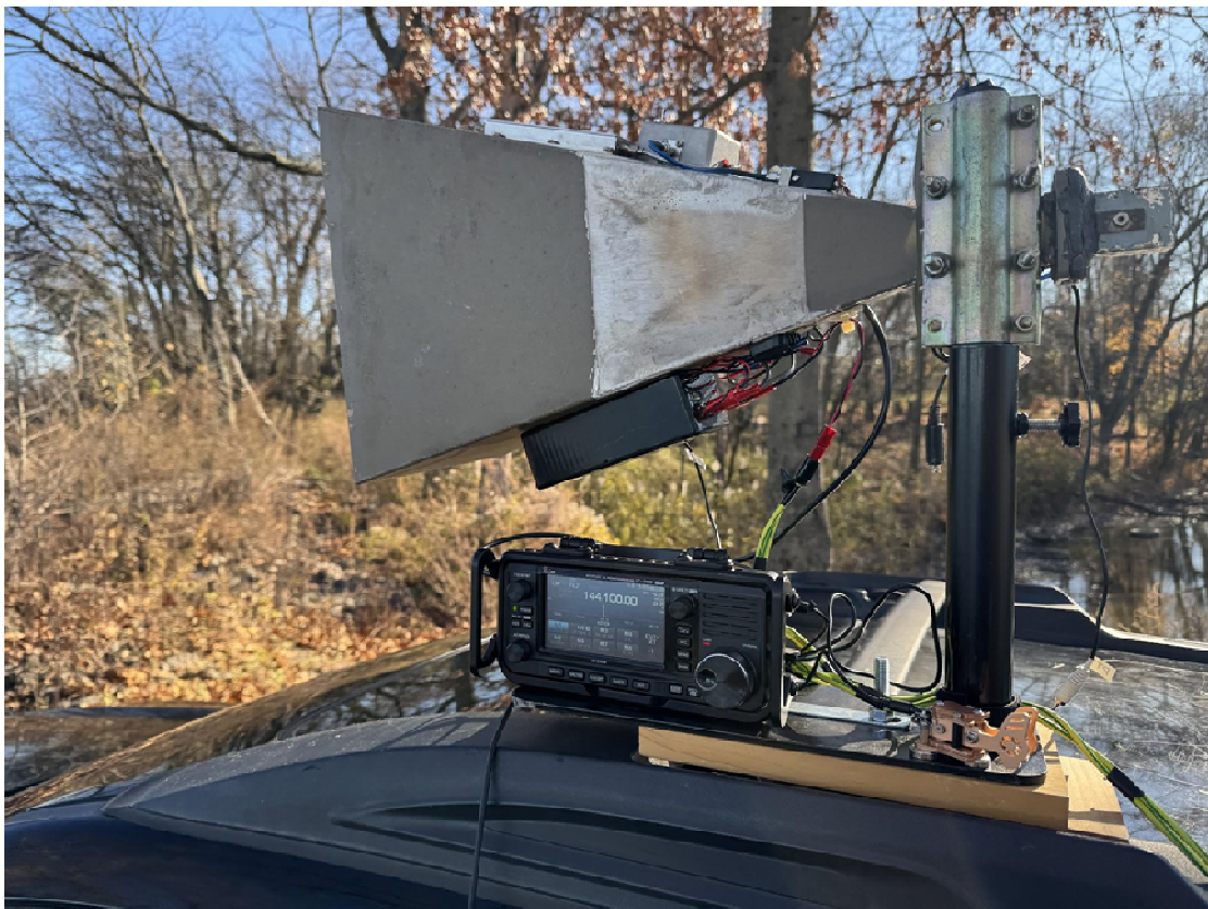
5.7 GHz Horn is mounted on a quick mount for pointing on the Subaru Outback, all components are mounted directly to the horn, including the transverter, power amp, pre-amp and switching relays and the Transmit / Receive Sequencer. The horn is removed during travel and mounted as I reach the over-look areas.
