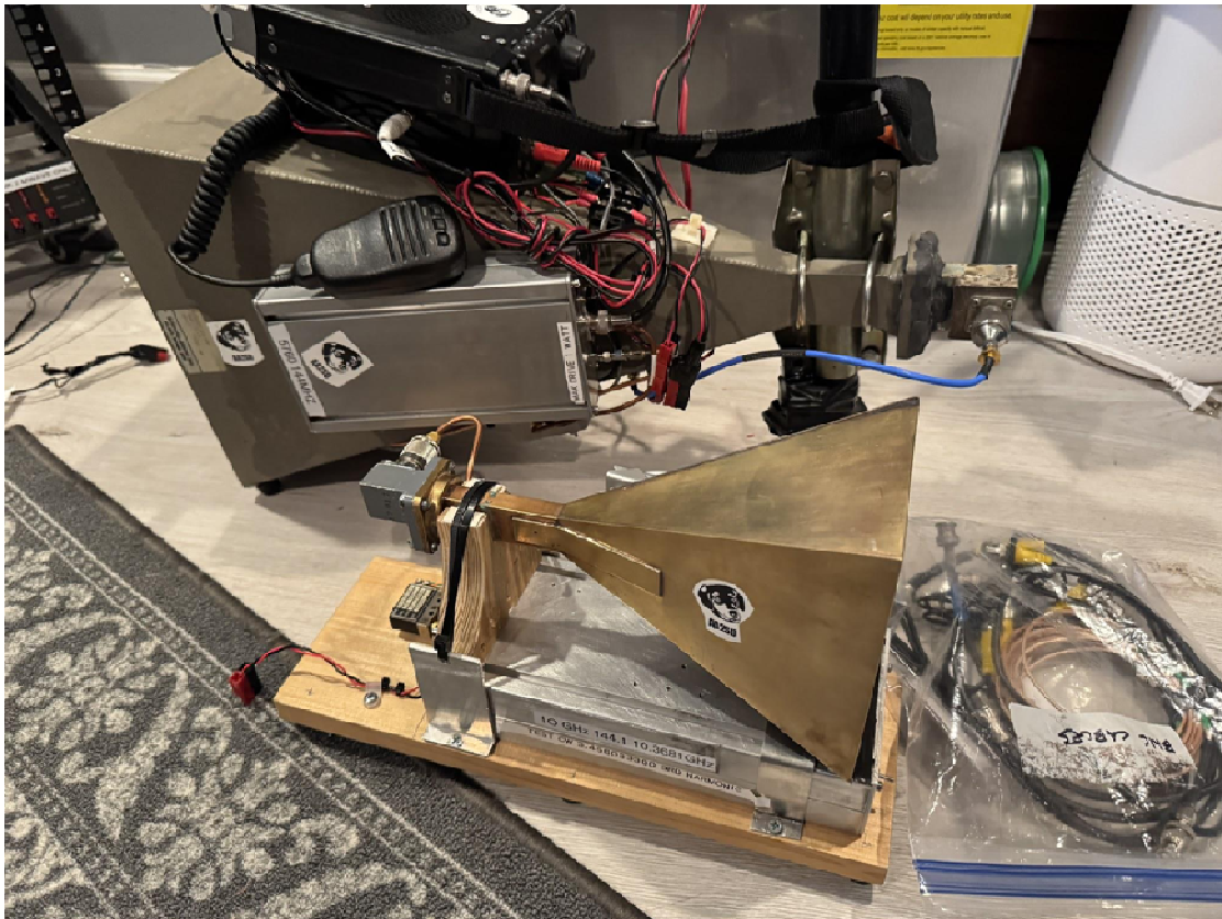
Ray N3RG created the shoe-shine box set up for both horns with quick deployment as a Rover
